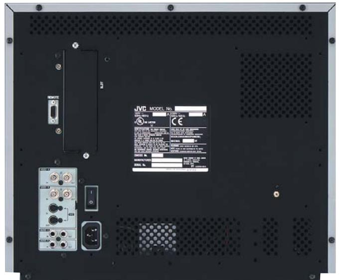
This photograph shows the rear panel with no optional input card fitted. The blanking plate, which covers the card slot and which is attached by two screws, can be seen between the monitor's reference plate and the 15-pin D-sub remote control socket.
